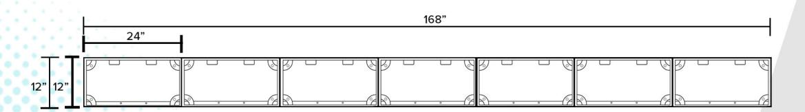
Must lift final assembled sign with a minimum of two lifting points. 330 maximum lbs per lifting pin.
