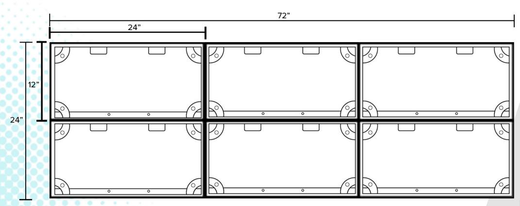
Must lift final assembled sign with a minimum of two lifting points. 330 maximum lbs per lifting pin.
