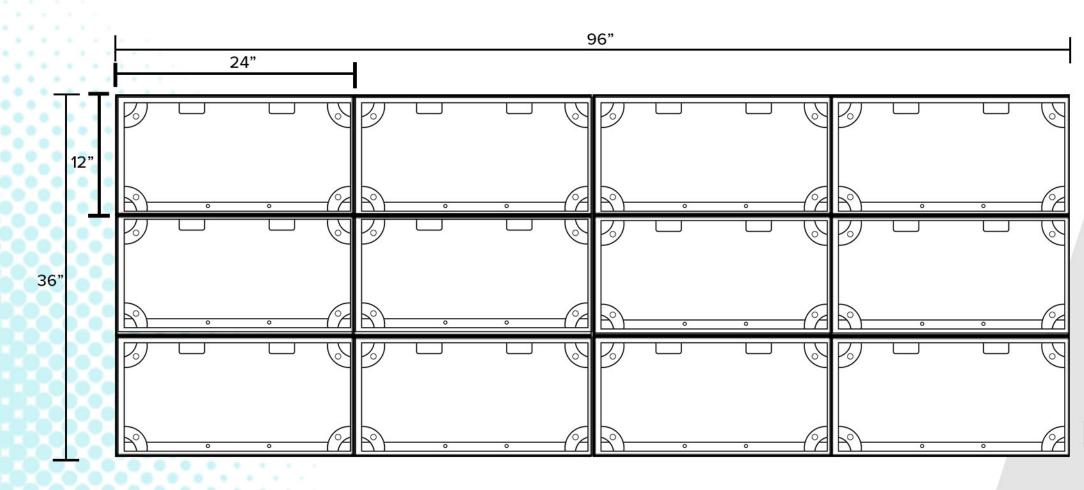
Must lift final assembled sign with a minimum of two lifting points. 330 maximum lbs per lifting pin.
