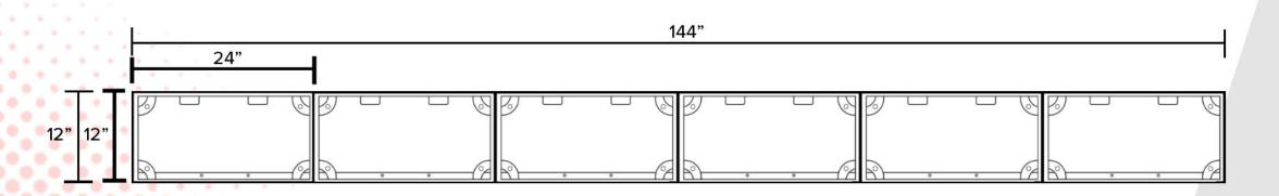
Must lift final assembled sign with a minimum of two lifting points. 330 maximum lbs per lifting pin.
