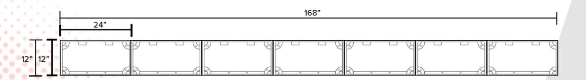
Must lift final assembled sign with a minimum of two lifting points. 330 maximum lbs per lifting pin.
