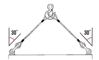
Must lift final assembled sign with a minimum of two lifting points. 330 maximum lbs per lifting pin.
